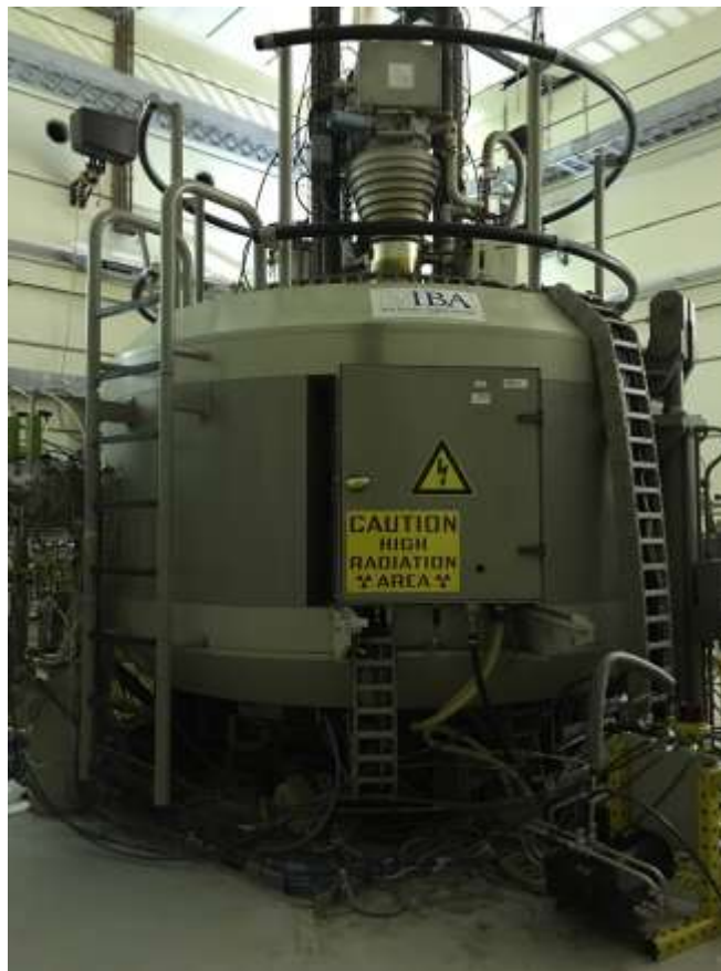
Fig. 1: The IBA 30 Cyclotron within the vault
